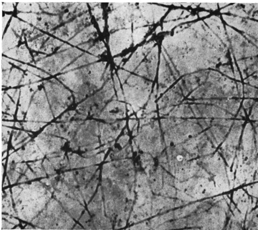
Figure 3—Electron micrograph of softwood cellulose microfibrils stained with Ag + , unshadowed. Magnification: ca. 25 000 ×, reproduced without reduction
