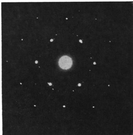
Figure 4 —Electron diffraction pattern given by a polyethylene single crystal (Keller 2 )
