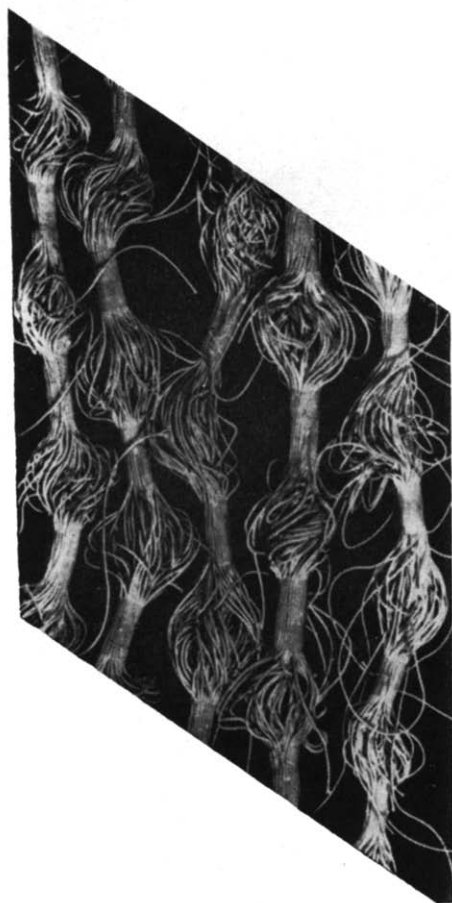
Figure 36—The model of stretched polyethylene after Statton and Geil 29
