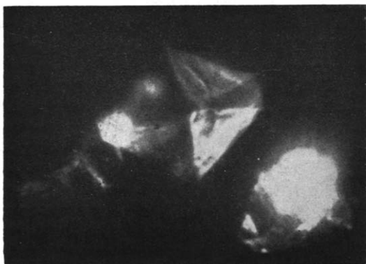
Figure 10 —Dark field optical micrograph of a monolayer polyethylene crystal while floating in suspension. The pyramidal nature of the crystal is revealed. Magnification \times 800 ; reproduced without reduction. (Bassett, Frank and Keller, in preparation)
