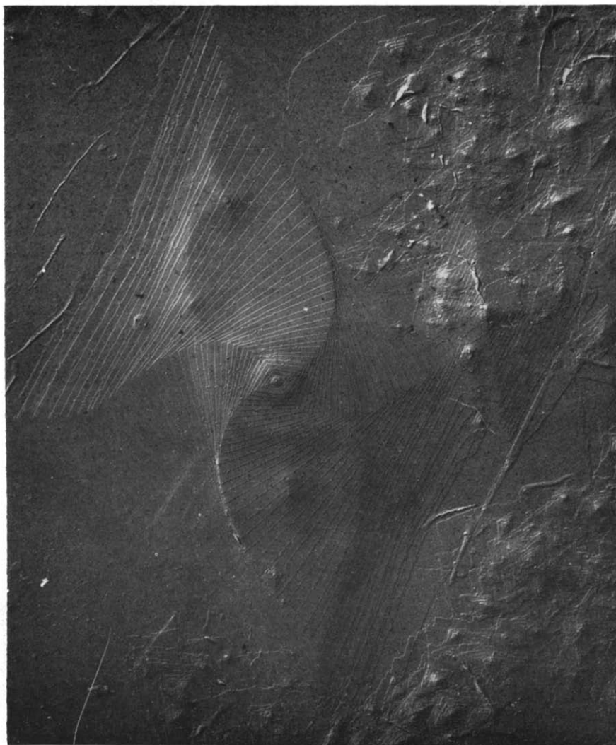
Figure 14—Multilayer polyethylene crystal where consecutive terraces are rotated with respect to each other always by the same amount in the same sense. Electron micrograph, replica, magnification \times 6000 ; reduced \times 3/4 on reproduction. (Bassett, Keller and Mitsuhashi, unpublished)
